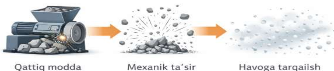
Rasm 1. Mexanik dispersiya jarayonida chang hosil bo'lishi
