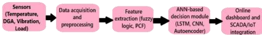
Fig. 1. Architecture of the proposed ANN-based online monitoring system.
