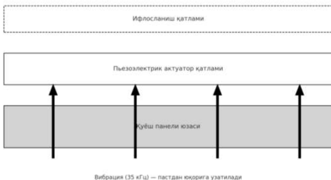
2-rasm. Pyezoelektrik tozalash tizimining 2D sxemasi
